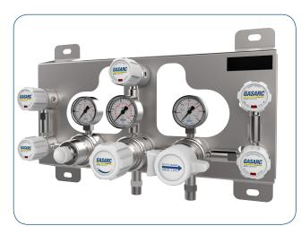
The Spec Master HPD6040 Series two stage differential autochange control panels are designed for primary pressure gas control of non-corrosive or toxic, high purity gases up to grade 6.0 purity (99.9999%), on gas distribution systems where constant delivery pressure is required.
